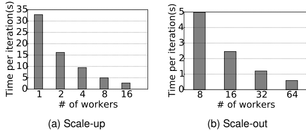
Fig. 11. Scale-up and Scale-out for PageRank on Twitter Graph communication phase (for the SVDPP case), this means the communication can not be fully masked by computation. For PageRank, in our computer cluster, communication can be fully overlapped by computation.
