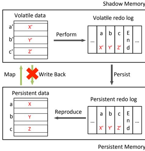
Fig. 1. DuDETx memory architecture and data movement in the three steps. Data X, Y and Z locate at addresses a, b and c in the persistent memory, respectively. These addresses are mapped to a', b' and c' in the shadow memory.
