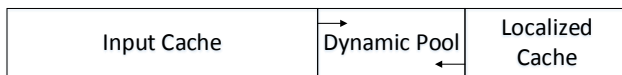
Fig. 5. The whole cache space is divided into three parts, namely Input Cache, Dynamic Pool and Localized Cache. Blocks in Dynamic Pool are used on demand as Input Cache or Localized Cache depending on the workload to get the most benefit of caching.
