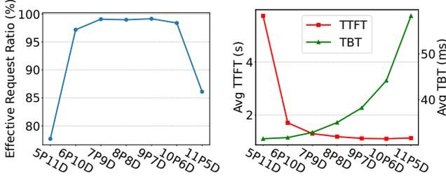
(a) Effective request capacity with varying P/D ratio. (b) Latency with varying P/D ratio.
