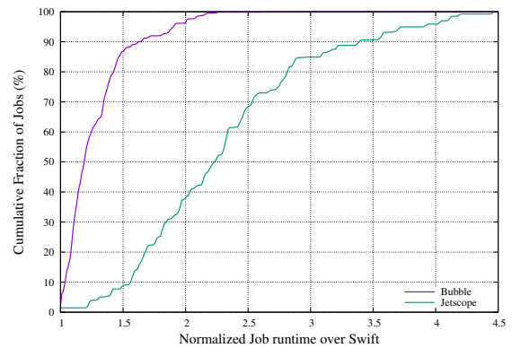
Fig. 11. Normalized execution latency of 2,000 jobs with JetScope, Bubble Execution, and Swift on the 100-nodes cluster.
